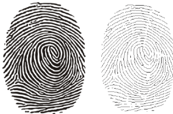
Figure 7: Finger print before and after binarization
